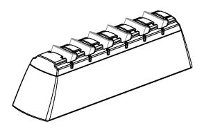
The Companion Group Charger accepts up to six battery packs for charging. Each slot has a LED indicator. Batteries are charged independent of position. For example, the first battery inserted is the first battery charged.
