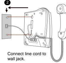
Place the telephone onto the wall mount plate and slide it down.
